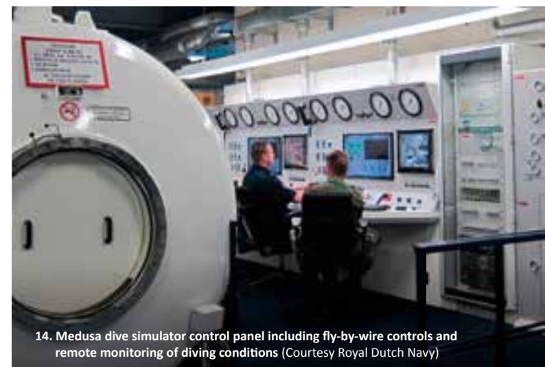
13. Control apparatus outside of the hyperbaric evacuation chamber, which enables the life-support crew to control the living environment of the divers
